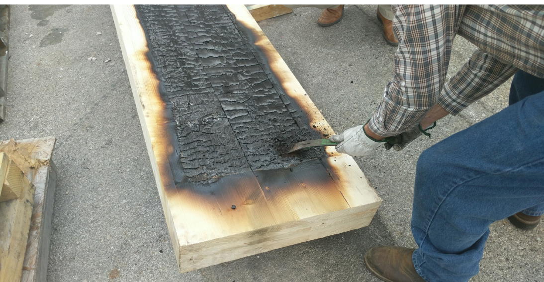
In addition to passing the required furnace testing, Katerra CLT is tested for spread of flame and smoke index ratings.
