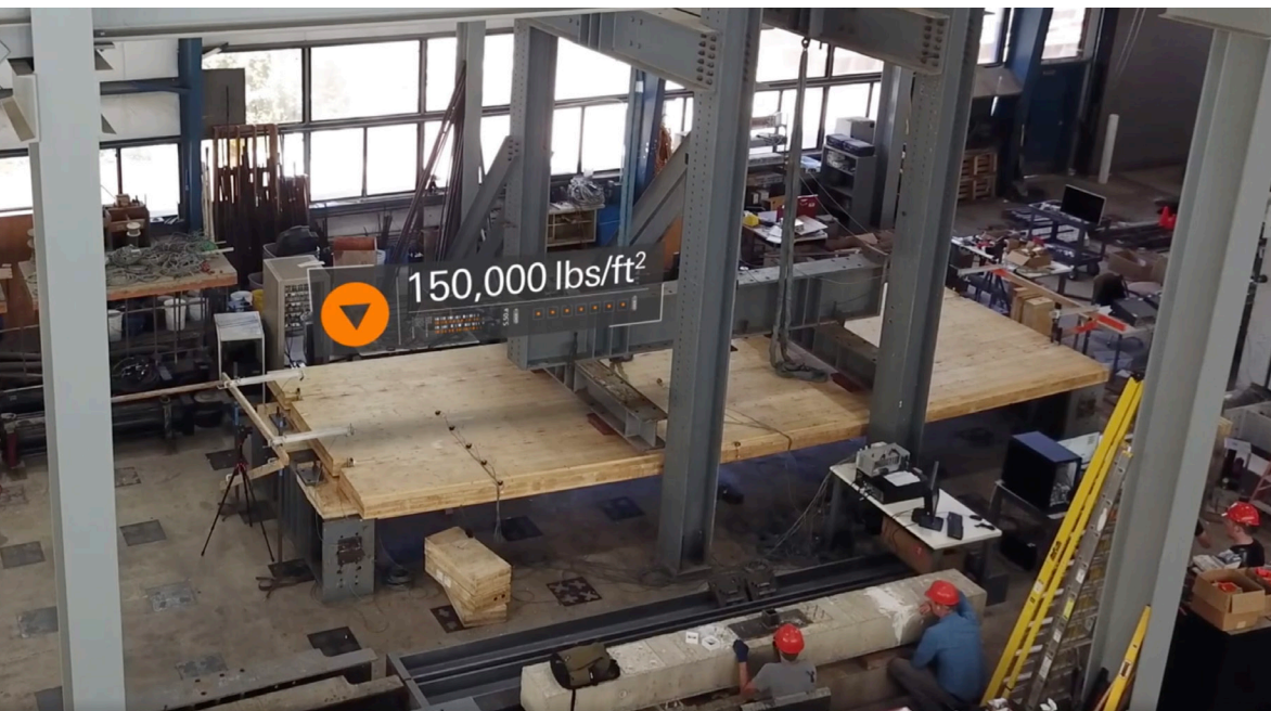
Over 400 specimens of Katerra cross-laminated timber products have been individually tested to ensure they are structurally-sound.
