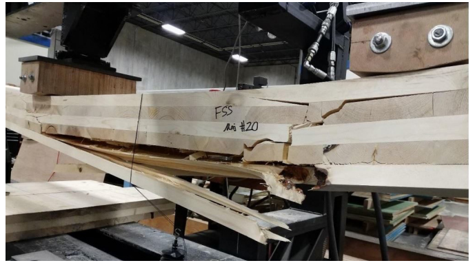
Flatwise flexural strength testing (top) and edgewise shear strength testing.
